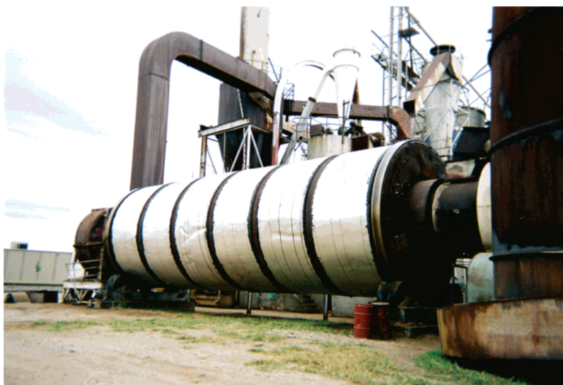
FIGURE 2. Large-scale drying of the biomass occurs within 5 h of harvesting and can produce up to 100 tons of dried plant material per day.
